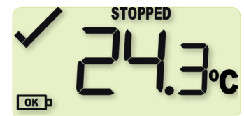
Figure 19: HAXO-16BT display while the user is pressing the START button, REC• disappeared
