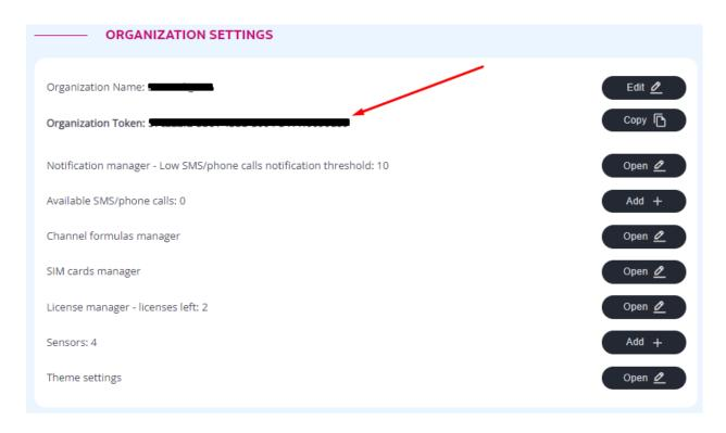
Organization token should be entered in the *Token* field in the Efento Gateway configuration page (Settings > Server). After entering the Organization token, measurements from all sensors within the Gateway's range will be automatically sent to the Efento Cloud platform.
