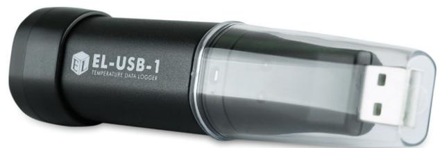
This standalone data logger measures and stores more than 16,000 temperature readings over a -35 to +80°C (-31 to +176°F) range with a resolution of 0.5°C (1°F).
