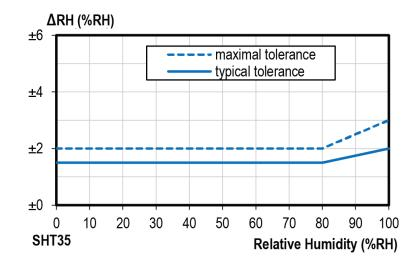
Typical tolerance of RH over Temperature:
